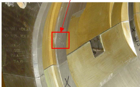
Fig. 7 Damage on Bearing 3 surface
