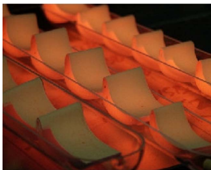
Fig. 2 Arrangement of sample in quartz boats for daily cycling in the furnace
