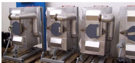
Fig. 8 Primary-surface recuperators ready to be installed in T100 machines (courtesy of Turbec)
